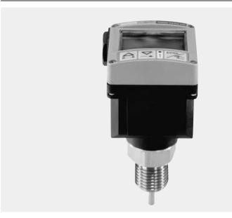
This Sensor/Switch is specially designed to switch a valve, pump, heaters, etc... and establish an ON/OFF control loop. The switching point can be programmed with the 3 key pads on the display or externally from a programmable logic controller via a 4-20 mA loop. Additionally, the process value can be transmitted to the PLC (4-20 mA). The connection to the process in the piping is done with standard fittings.
