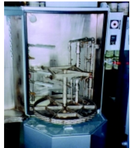
(3) Model 2012 12" (30cm) Standard Air Knives perform the drying cycle in this parts washer.
