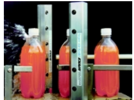
(2) Model 110012 12" (30cm) Super Air Knives blow water off bottles prior to labeling.
