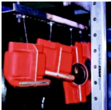
A Model 110018 18" (46cm) Super Air Knife cools molten plastic following dip molding.
