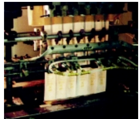
A Model 2012 12" (30cm) Standard Air Knife opens mustard packets prior to fill.
