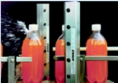
Bottles exiting a washer are blown dry by (2) Model 110012 12" (30cm) Super Air Knives prior to labeling.
