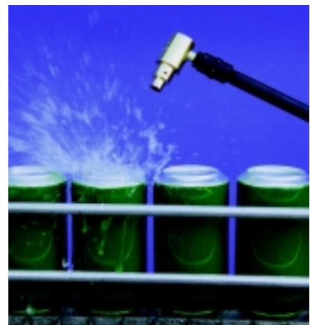
A Model 6013 High Velocity Air Jet dries cans prior to ink jetting the date code.
