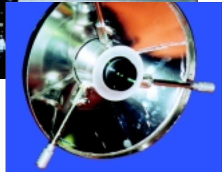
Special high temperature vortex tubes keep a boroscope lens cool while inserted into a 1200°F boiler porthole. (front view)
