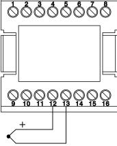
Figure 2.5 Thermocouple Input Wiring
