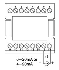
Figure 2.10 Input 2 Linear Current Wiring
