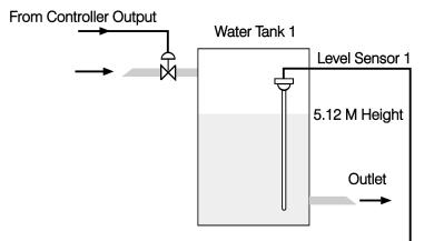
Figure 5.13 Differential Control Example
