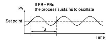
Figure 3.24 Critical Steady State
