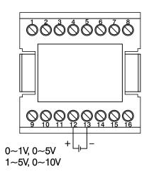
Figure 2.7 Input 1 Linear Voltage Wiring
