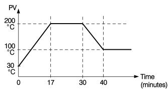
Note: When the ramp function is used, the lower display will show the current ramping value. However it will revert to show the set point value as soon as the up or down key is touched for adjustment. The ramping value is initiated to process value either power up or RAMP and /or set point are changed. Setting RAMP to zero means no ramp function at all.
