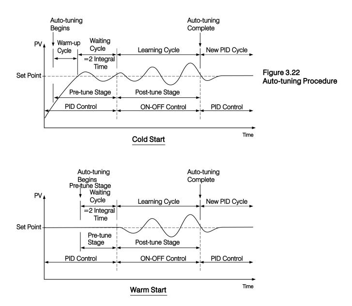
If the auto-tuning begins near the set point (warm start), the unit passes the warm-up cycle and enters the waiting cycle. Afterward the procedures are same as that described for cold start.
