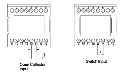
Figure 2.13 Event Input Wiring
