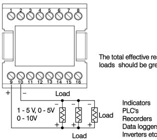
The total effective resistance of parallel loads should be greater than 10K Ohms.
