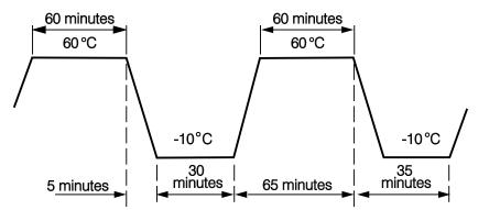
Figure 5.9 Temperature Profile of Chamber
