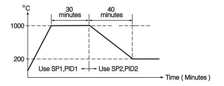
Figure 5.16 Dual Set Point /PID Profile
