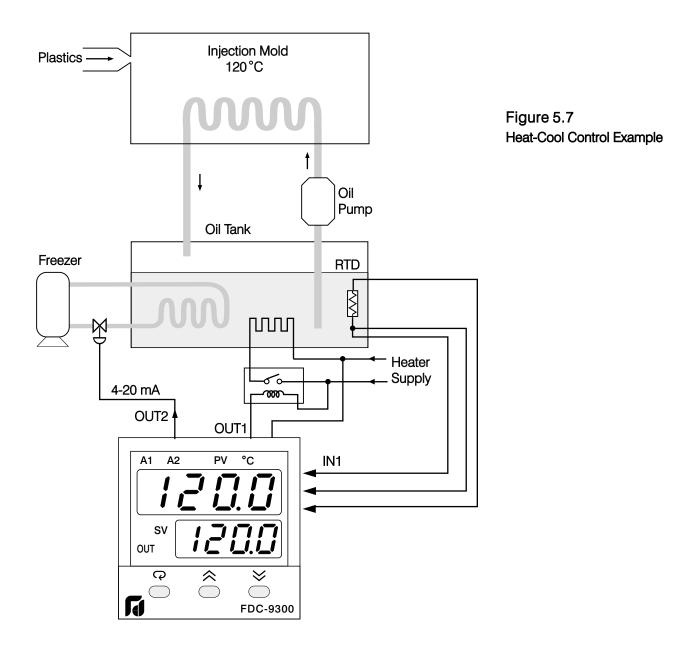
The PID Heat-Cool is used for the above example. To achieve this set the following parameters in the Setup Menu:
