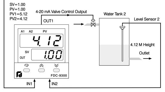
Adjust SP1(here is 1.00) to control the difference between PV1 and PV2. Choosing P1-2 for PVMD, the PV display will show the difference value (PV1-PV2) between PV1 and PV2, and this value will be stabilized to the set point ( here is 1.00).
