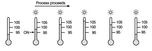
Figure 3.14 Latching Deviation Band Alarm
