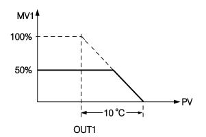
Figure 4.5 Power Limit Function
