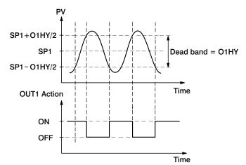
Setup ON-OFF :  $OUT1 = \boxed{r \not E \ \ r}$ PB1 = 0 Adjust :SP1, O1HY, TIME( if enabled)
