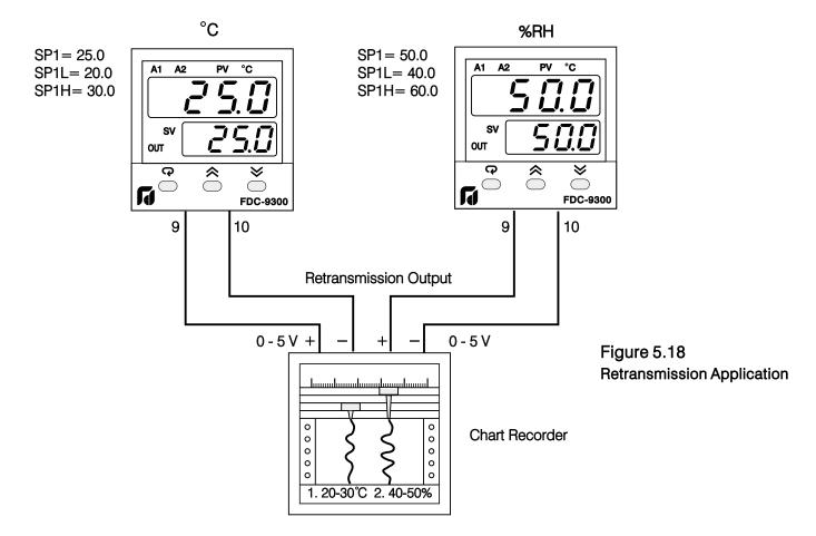
SP1L and SP1H are used to limit the adjustment range of set point.
