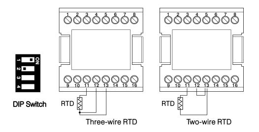
Figure 2.6 RTD Input Wiring
