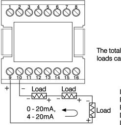
The total effective resistance of serial loads can't exceed 500 ohms.
