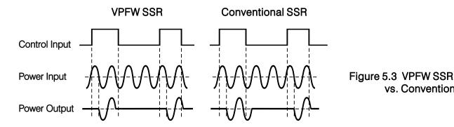
The VPFW switches the load without DC current, hence minimize the harmonic current and stress on the load. The load life is prolonged.
