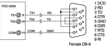
Figure 2.21 Configuration of RS-232 Cable
