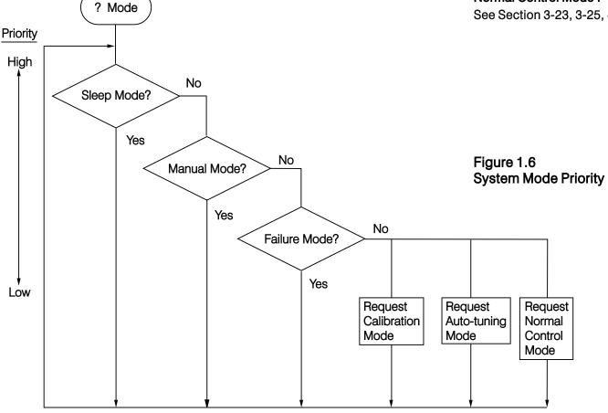
The calibration mode, auto-tuning mode and normal control mode are in the same priority level. The sleep mode is in the highest priority.
