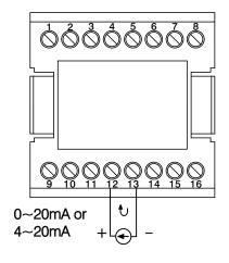
Figure 2.8 Input 1 Linear Current Wiring
