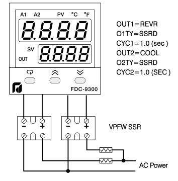
Figure 5.4 VPFW SSR Application Example
