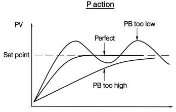
Figure 3.25 Effects of PID Adjustment
