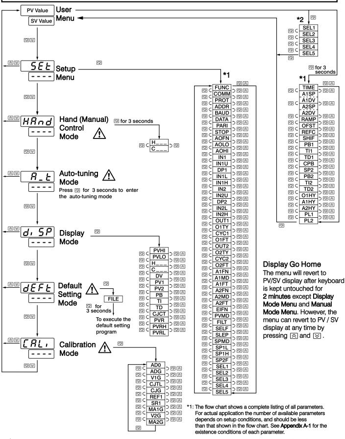
Apply these modes will break the control loop and change some of the previous setting data. Make sure that if the system is allowable to use these modes.
