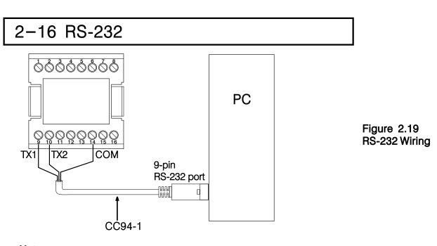
**Note:** If the FDC-9300 is configured for RS-232 communication, the EI (Event Input) is disconnected internally. The unit can no longer perform event input function (EIFN).
