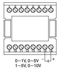
Figure 2.9 Input 2 Linear Voltage Wiring
