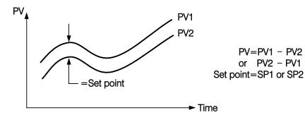
Figure 4.4 Relation between PV1 and PV2 for a Differential Control
