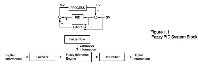
The function of Fuzzy Logic is to adjust PID parameters internally in order to make manipulation output value MV more flexible and adaptive to various processes. The Fuzzy Rule may work like these:
