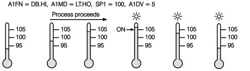
Figure 3.16 Latching /Holding Deviation Band Alarm
