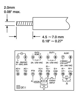
Figure 2.2 Lead Termination
