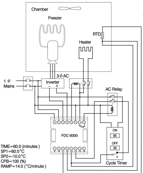
Figure 5.8 A Temperature Cycling Chamber
