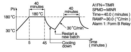
Figure 5.11 Temperature Profile of Baking Oven
