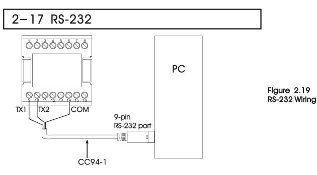
Note: If the FDC-9300 is configured for RS-232 communication, the El (Event Input) is disconnected internally. The unit can no longer perform event input function (EIFN).
