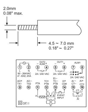
Figure 2.2 Lead Termination
