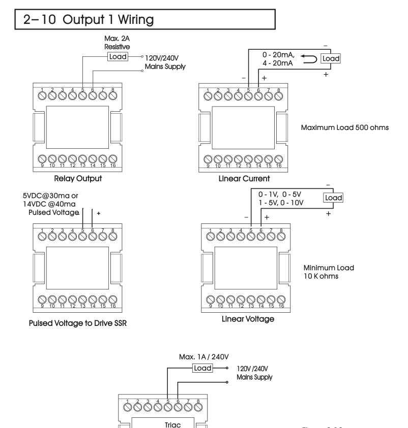
Figure 2.12 Output 1 Wiring
