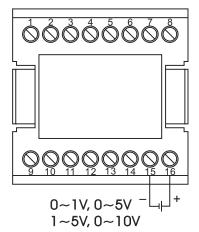
Figure 2.8 Input 1 Linear Current Wiring
