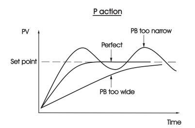
Figure 3.7 Effects of PID Adjustment
