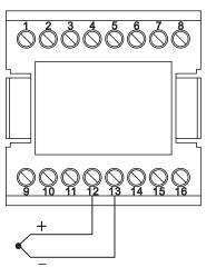
Figure 2.5 Thermocouple Input Wiring
