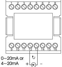
Figure 2.10 Input 2 Linear Current Wiring
