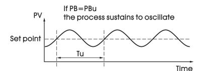
Figure 3.6 Critical Steady State
