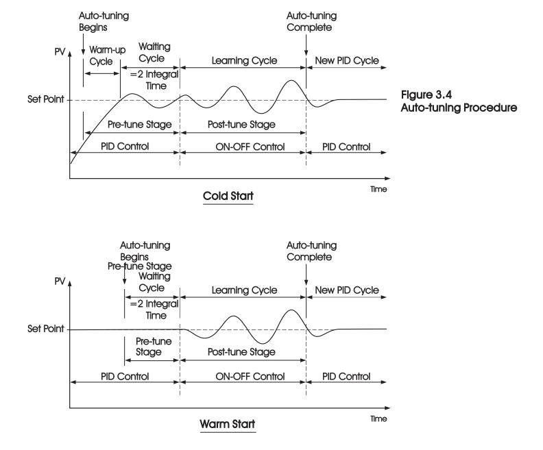
If the auto-tuning begins near the set point ( warm start ), the unit passes the warm-up cycle and enters the waiting cycle. Afterward the procedures are same as that described for cold start.
