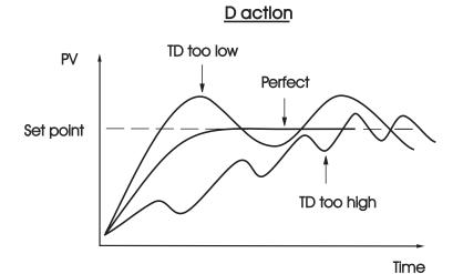
Figure 3.8 (Continued) Effects of PID Adjustment
