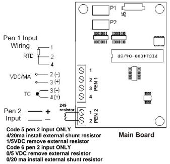
Fig. 2.6 Two Pen Universal and Thermal Inputs
