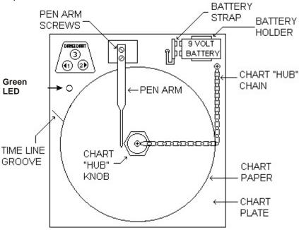
Figure 2.10 Recorder Platen Layout/Battery Installation
