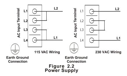
The recorder uses AC power when it is operating normally. The battery back-up option on ink recorders will allow the recorder to operate for approximately 48 hours in case of a power loss. AC input can be fused with a 250VAC, .5 Amp fuse.
