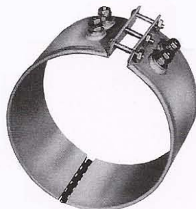
Fig. 12: Hinged Half-Band—convenient where two piece heaters are required. Shown with Fig. 8 mounting flange and T2 screw terminals. Available with any termination or mounting arrangement.
