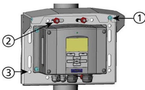
Figure 12 Mounting the Rain Shield with Installation Kit
