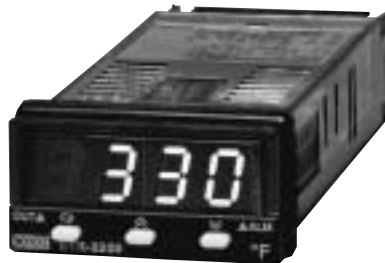
DISPLAY AFTER INPUT SHIFT. ADJUST SET POINT TO 330
