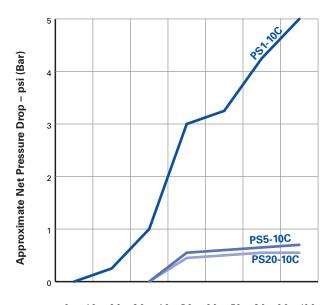
0 1.0 2.0 3.0 4.0 5.0 6.0 7.0 8.0 9.0 10.0 (3.8) (7.6) (11.4) (15.1) (18.9) (22.7) (26.5) (30.3) (34.1) (37.9) Flow Rate – gpm (Lpm)
