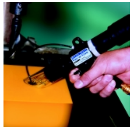
Model 6394 Deep Hole Vac-u-Gun All Purpose System removes the chips from a drilled plastic part.
