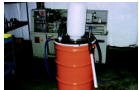
Chips can be vacuumed directly to separate drums for recycling.
