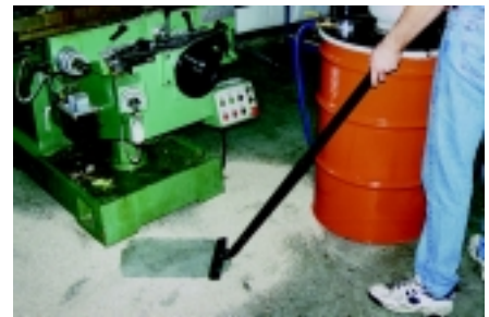
Room air remains dust free as the Chip Vac removes dusty absorbent.
