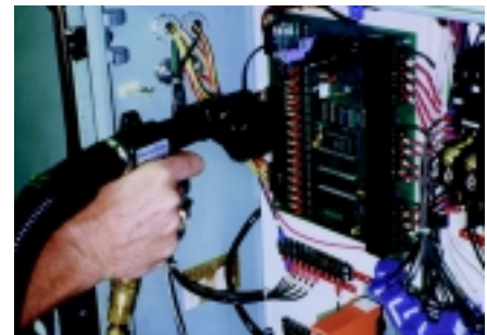
Model 6292 Vac-u-Gun Transfer System carries dust away from sensitive electronic controls.
