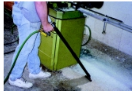
Model 6192 Vac-u-Gun Collection System with bag, vacuums absorbent and chips.
