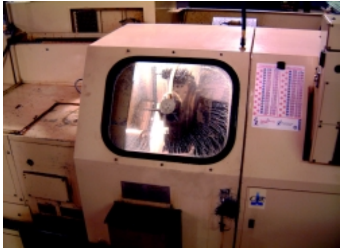
When compressed air is turned on, the Model 6200 Air Disk Window Blowoff keeps the part and process visible.
