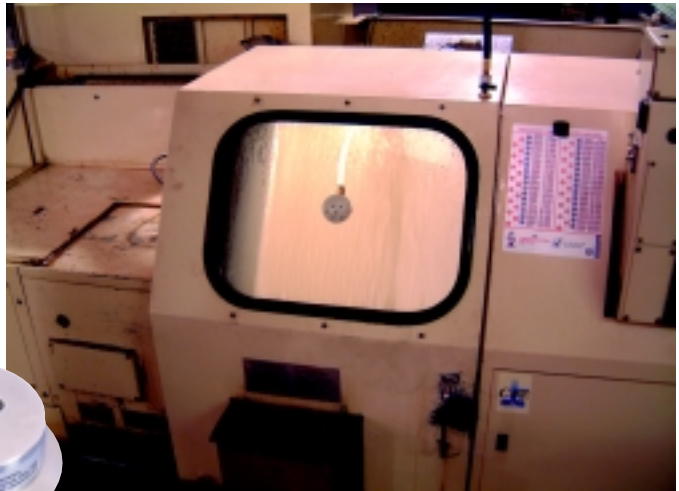
When the Air Disk Window Blowoff is off, the view is completely blocked.
