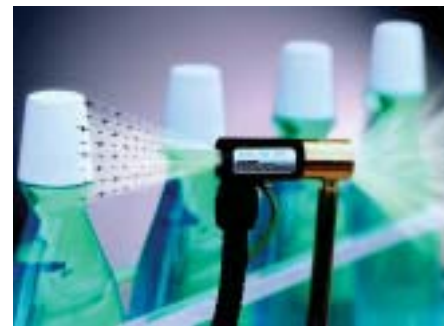
The Model 7294 Ion Air Jet and Power Supply neutralize and clean mouthwash bottles before installing the tamper-proof seal.
