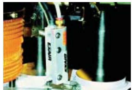
A Model 7103 3" (8cm) Standard Ion Air Knife removes dust from computer hard disks prior to assembly.
