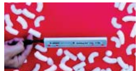
A Model 7006 6" (15cm) Ionizing Bar eliminates the static charge that causes packing peanuts to cling.
