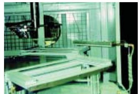
A Model 7212 12" (30cm) Standard Ion Air Knife System cleans metal frames prior to powder coating.
