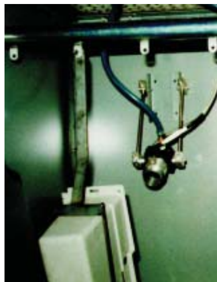
A Model 7292 Ion Air Cannon System removes static and dust from glove box inserts prior to flocking or painting.
