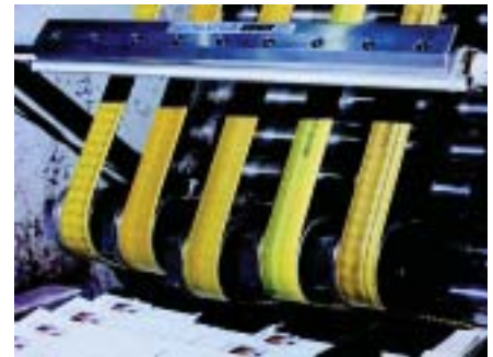
A Model 111118 18" (46cm) Super Ion Air Knife prevents jamming on a stacker.
