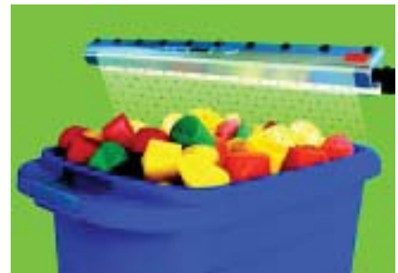
The Model 7218 18" (46cm) Standard Ion Air Knife System showers parts with static eliminating ions to prevent personnel shocks.
