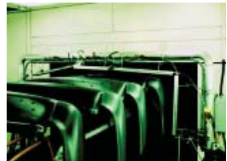
Bumpers, car bodies and fascia are cleaned of dust and fibers prior to painting.
