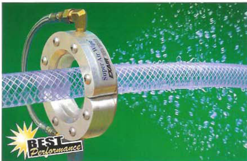
The Super Air Wipe uniformly dries a hose as it exits a bath.
