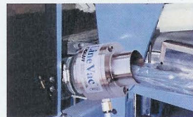
The Model 6084 2" (51mm) Line Vac transports scrap trim to a waste barrel.
