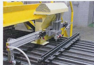
(2) Model 6083 1-1/2" (38mm) Line Vacs convey reject metal caps from a fluorescent lamp operation to a scrap bin.
