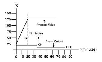
The dwell function may be used to operate an external device such as a siren to alert when a soak time has been reached.
