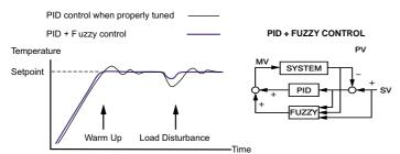
In addition, this instrument has functions of single stage ramp and dwell, auto-tuning and manual mode execution. Ease of use is also an essential feature with it.
