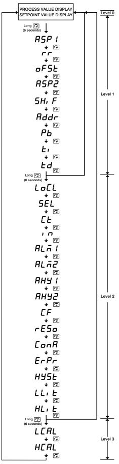
The "return" key can be pressed at any time. This will prompt the display to return to the Process value/Setpoint value. Power Applied:
