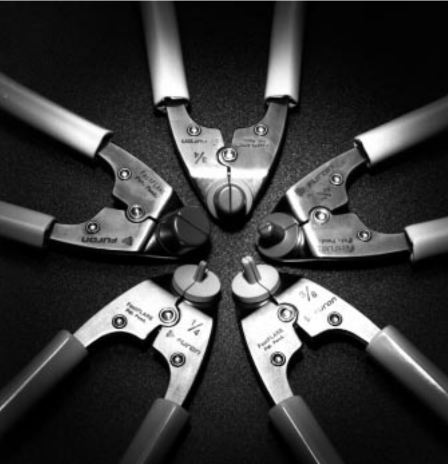
Furon FastFLARE forming tools are ideal for cold flaring PFA tubing. For use with Furon Flare Grip® and Flare Grip II PFA fittings.
