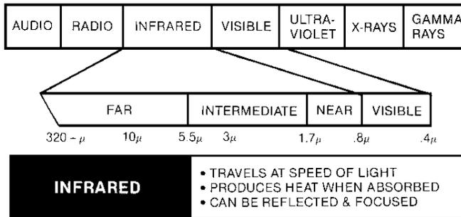
The basic infrared theory is that the intermediate heating of the air between the heat source and the product is not required. Because radiant energy travels at the speed of light, heat transfer is very efficient when the characteristics of the material being heated absorbs infrared well. Also, the energy can be directed into specific patterns by the use of reflectors.
