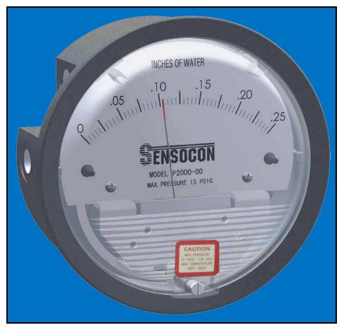
The Series P2000 is a low cost, diaphragm operated, differential pressure gauge in an ABS housing. The P2000 can be used in applications for measuring positive, negative, or differential pressure with an accuracy of 2%. Standard applications include monitoring filter status, duct static pressure, room pressure, fan or blower pressure, paint booths, dust collectors, and cabinet purging along with many others.
