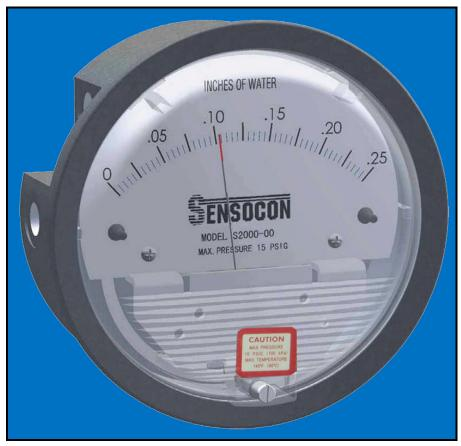
The Series S2000 is a low cost, diaphragm operated, differential pressure gauge. The S2000 can be used in applications for measuring positive, negative, or differential pressure with an accuracy of 2%. Standard applications include monitoring filter status, duct static pressure, room pressure, fan or blower pressure, paint booths, dust collectors, and cabinet purging along with many others.
